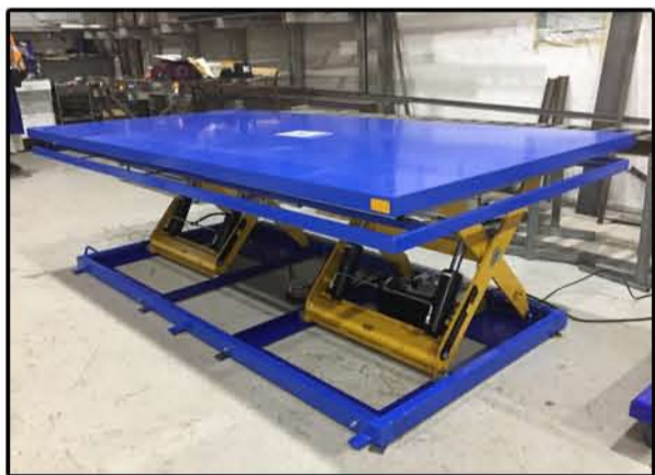
Custom LTH2010C dual scissor lift table
